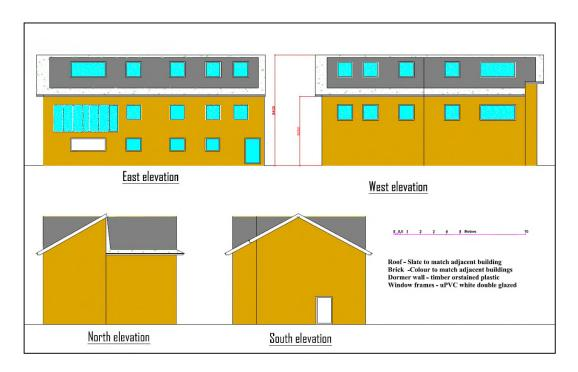
The building actually constructed involved a three storey flat elevation to Kingsway and incorporated a flat roof with a partial pitch facing into the site with four dormer windows, and blockwork was used on the elevations. This is indicated on the drawing below which was submitted to regularise the situation but subsequently withdrawn.
